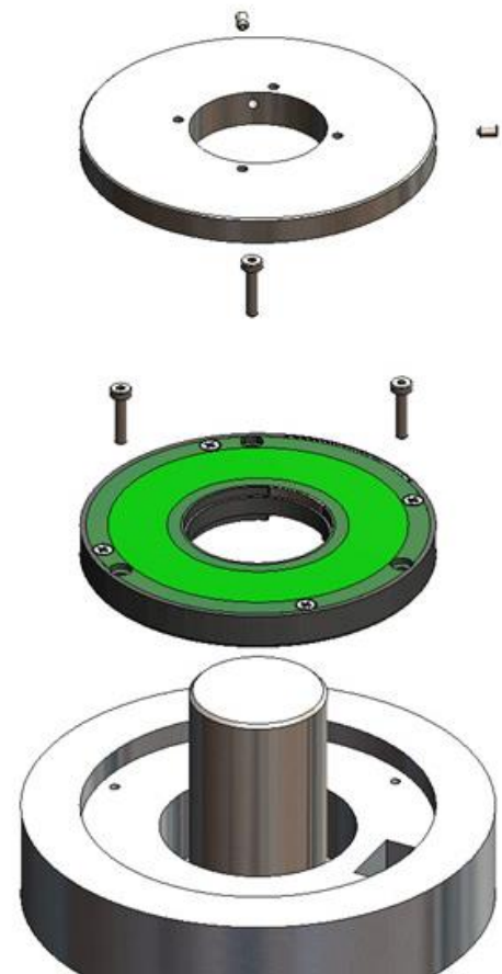
Figure 4: Hollow-Shaft Encoder Installation
